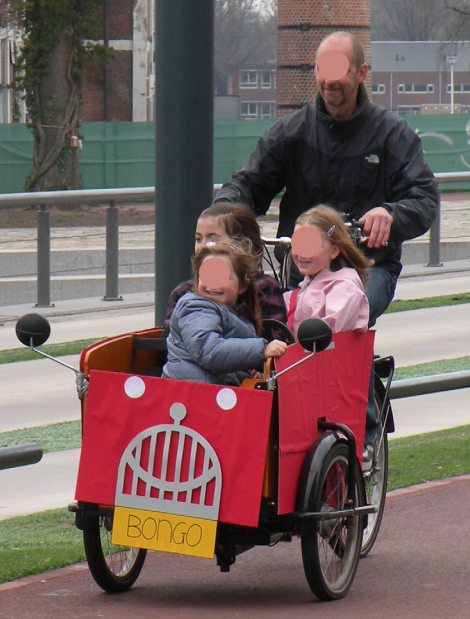
Figure 6.5: team 1 designed a carrier bike to rent to parents on holiday parks to transport their children in and around the park. The most important issues they worked on was to make the bike appealing for children so they could persuade their parents to rent the bike. Furthermore it should be comfortable to sit in and allow different positions for multiple children. Their final design had the appearance of a car and little play-steers for the children. Furthermore it had adjustable benches to allow the different positions
