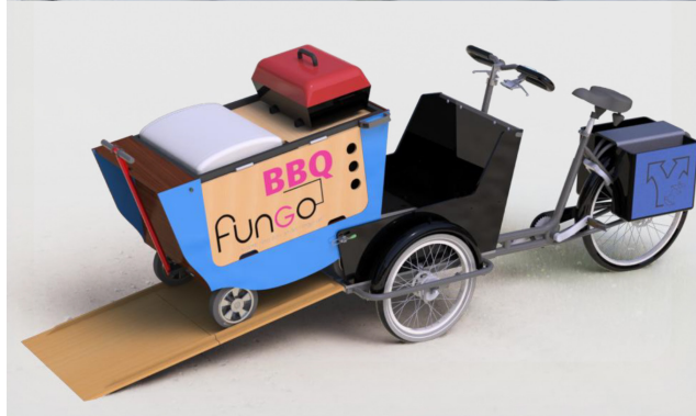
Figure 6.7: team 3 designed a carrier bike to rent to general visitors of holiday parks for specific purposes (themes) such as a party, a picnic or going to the beach. The main issues they worked on was to allow easy adjustment of the bike to another theme, make it easy to store and reach all necessary tools for the theme and easy loading and unloading. They designed a bike with detachable theme-boxes one could drive out of the main box.
